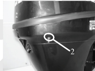
2. Cooling water checking hole
