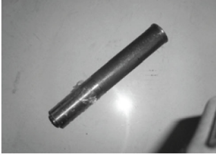
Drive shaft bearing installer
